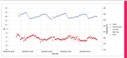
Two of our buoy deployable S1100 sensors were tested on the shore side using both our user controlled, data stream direct to the laptop system and our stand alone autonomous interface, with measurements taken every 15 mins for 3 days.
