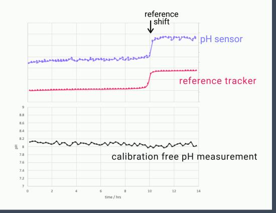
internal reference tracker looks out for any changes in the reference and accounts for this in-situ, making the measurement calibration free
